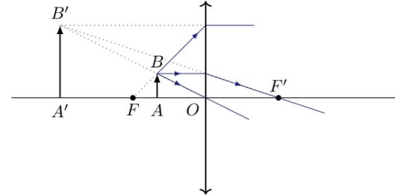
4.  $G_t = \frac{\overline{A'B'}}{\overline{AB}} = \frac{\overline{OA'}}{\overline{OA}} = \frac{f'}{f' + \overline{OA}} = 4$
